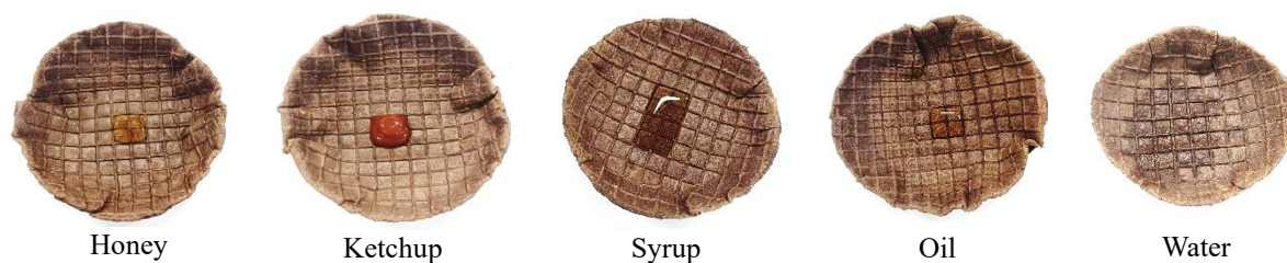
Fig. 5.18. Spreadability test of the biodegradable plates with different food models within 15 min
