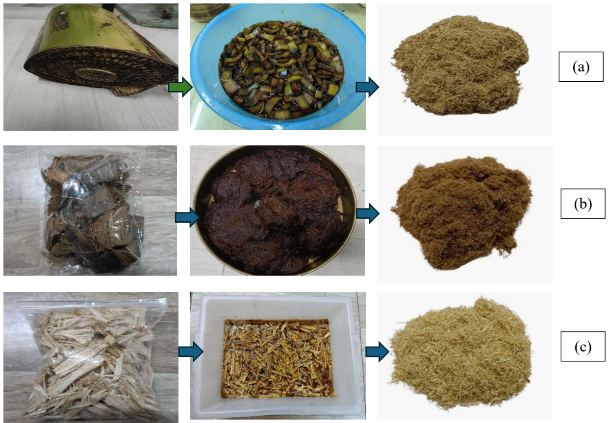
Fig. 5.1. Extraction of fibres from (a) raw banana pseudo-stem (b) raw coconut coir (c) raw sugarcane bagasse
