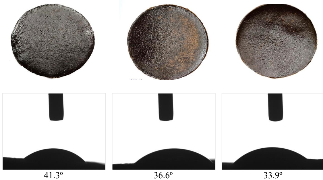
Fig. 5.16. Contact angle of biocomposites reinforced with plant fibres
