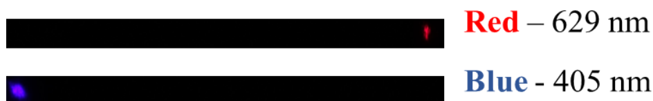
Figure 5.4. Spectral image of red and blue laser light obtained using the developed sensor.
