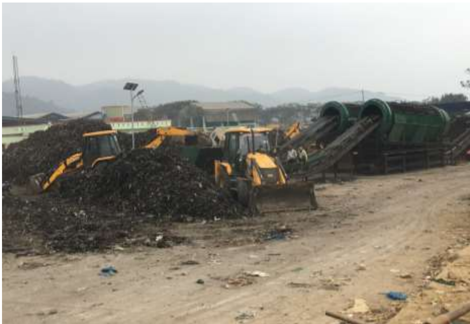
Image 19. Segregation of plastic and soil through a trommel being undertaken by GMC at the Boragaon dumping ground .
