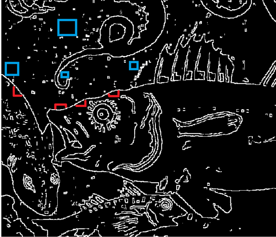
Figure 2-7: Adaptive windows for the median filter are designed using the generated edge-map ( E_r ).
