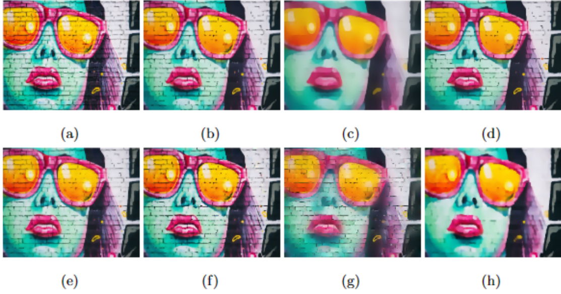
Figure 2-12: Comparative results for a brick wall graffiti image: (a) Original image and the filtered images produced by applying (b) BTF, k = 9, n_{itr} = 7 [32], (c) SATF ss = 7, sr = 0.05, st = 0.1, n_{itr} = 7, div = 30 [69], (d) RoG, \lambda = 0.01, \sigma_1 = 2, \sigma_2 = 4, K = 4, dec = 2.0 [22], (e) SATV, \lambda = 0.75 [125], (f) FABF \rho_{smooth} = 5, \rho_{sharp} = 5 [55], (g) RILS, \lambda = 0.75, \gamma = 50/255, n_{itr} = 25 [91], and (h) Proposed, W = 7 \times 7, n_{itr} = 7
