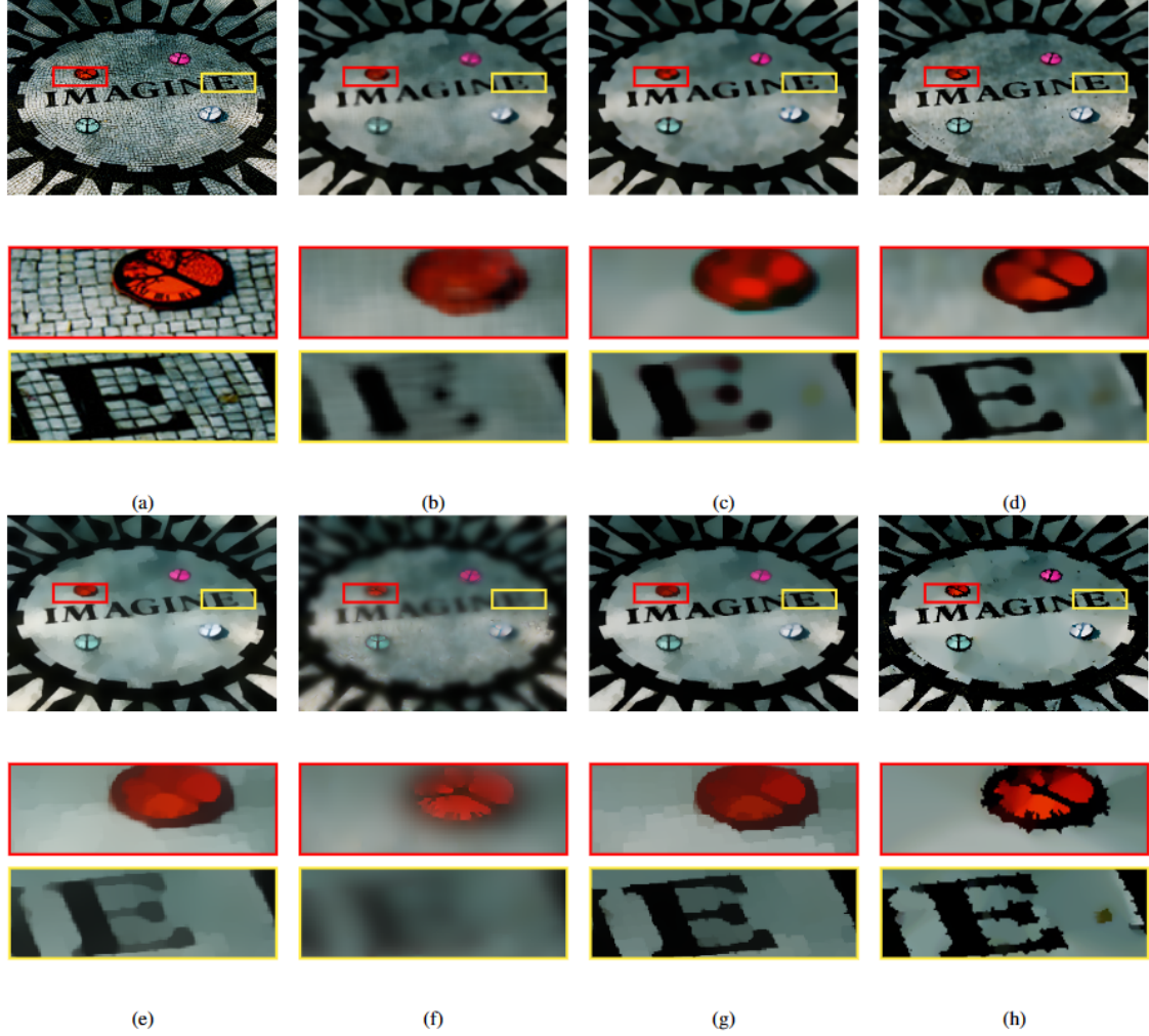
Figure 3-8: Comparative results of a mosaic floor image: (a) Original image and zoomed portions of it. Filtered images with best possible parameters and its respective SSIM Values obtained by (b) Reg-Cov ( k = 15, ps = 6, \sigma = 0.2 ) [SSIM = 0.36] [72] (c) BTF ( k = 9, n_{itr} = 7 ) [SSIM = 0.37] [32], (d) SATF ( ss = 3, sr = 0.1, st = 0.1, n_{itr} = 7, div = 30 ) [SSIM = 0.44] [69], (e) SATV ( \lambda = 1.25 ) [SSIM = 0.32] [125], (f) RILS ( \lambda = 1.5, \gamma = 50/255, n_{itr} = 15 ) [SSIM = 0.25] [91], (g) GISF ( \alpha = 0.75, \lambda = 1.25, n_{itr} = 10 ) [SSIM = 0.45] [92], and (h) Proposed ( w = 11 \times 11, n_{itr} = 5 ) [SSIM = 0.51] techniques.
