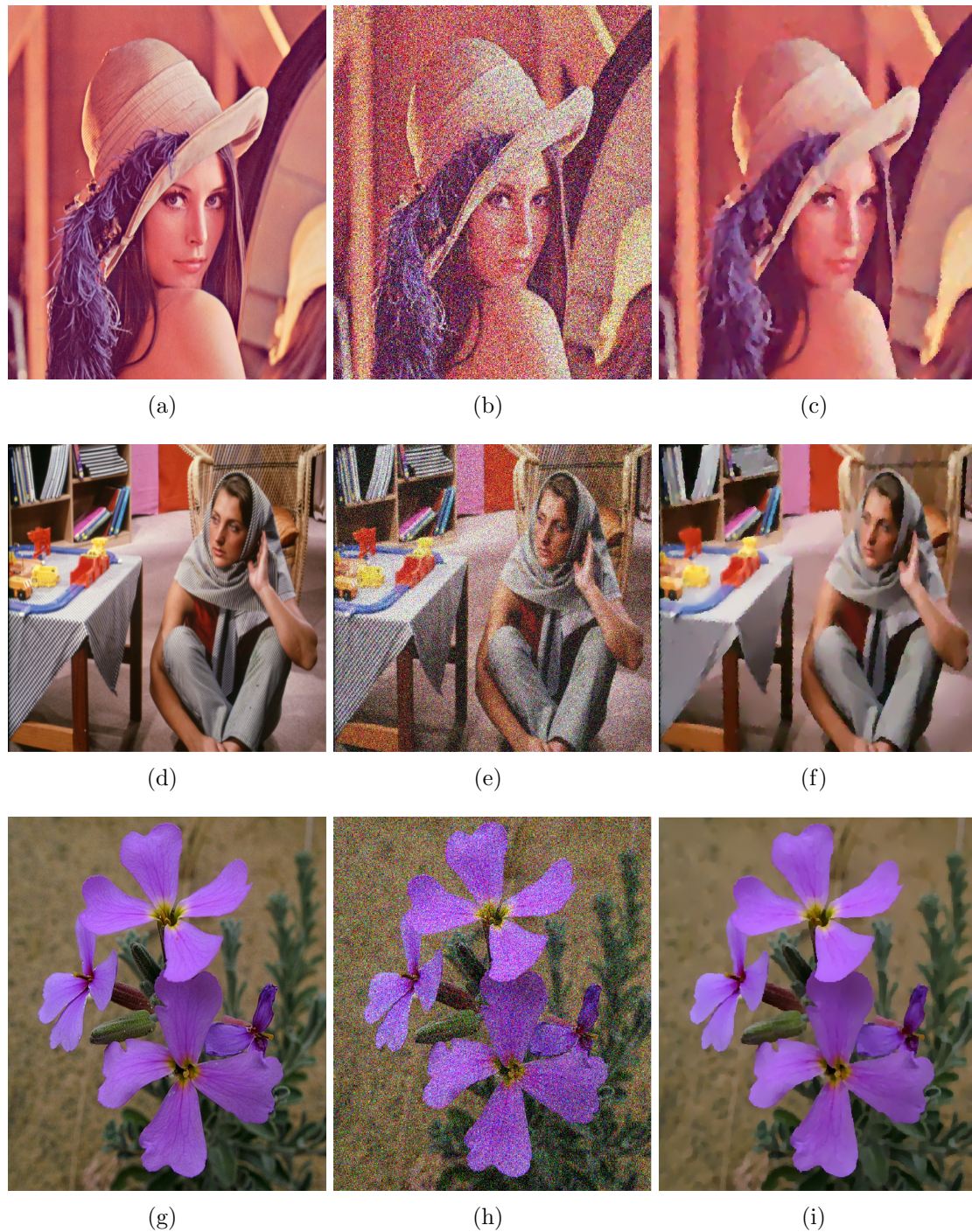
Figure 3-14: (a)(d)(g) Original images, (b)(e)(h) images with Gaussian noise ( \sigma = 0.03 ) and their corresponding (c)(f)(i) denoised images obtained by applying proposed filtering technique.
