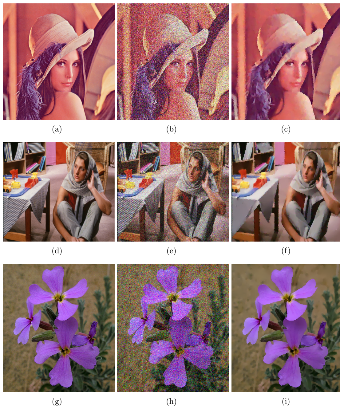
Figure 4-9: (a)(d)(g) Original images, (b)(e)(h) images with Gaussian noise ( \sigma = 0.03 ) and their corresponding (c)(f)(i) denoised images obtained by applying proposed filtering technique.
