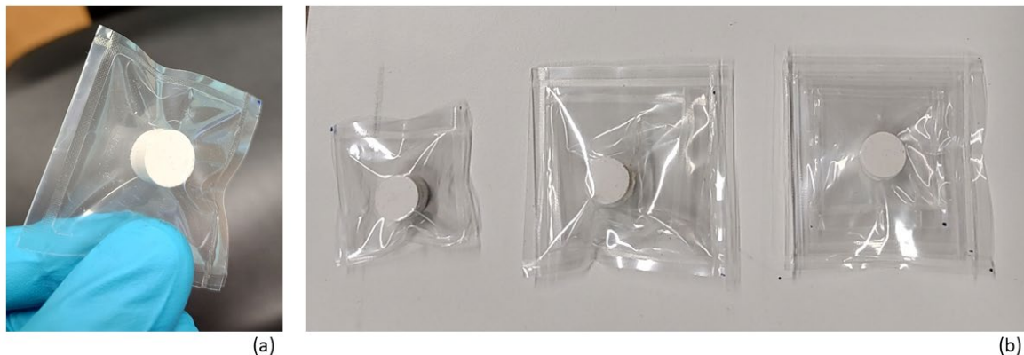
Figure 10: (a) A 1-layer pouch. (b) A 1-layer pouch, 2-layer pouch and 3-layer pouch (left to right).
