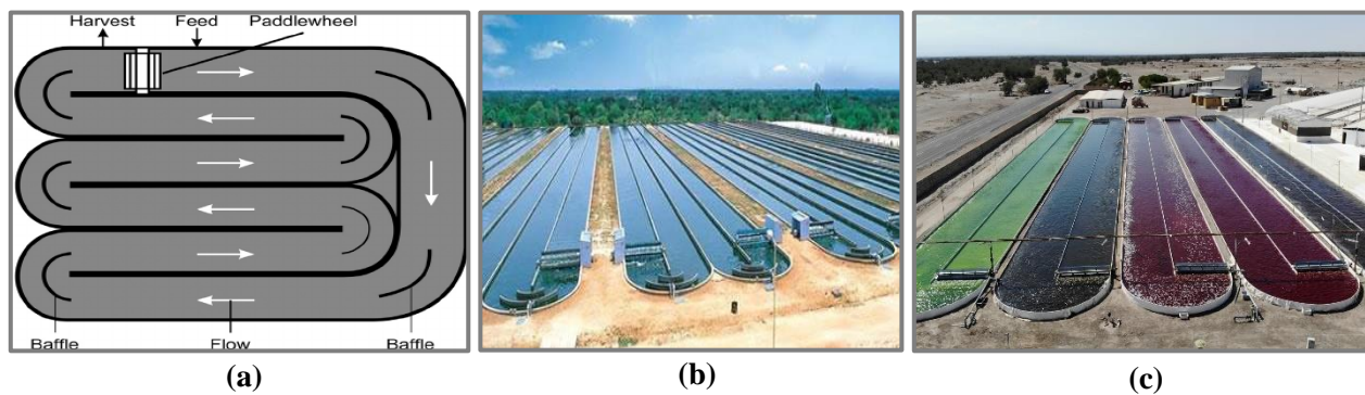
Figure 1.11 (a): Schematic of a raceway pond system, (b): Raceway pond system by Parry Nutraceuticals, India, (c): Raceway pond system Atacama Bionatural at Atacama Desert.
