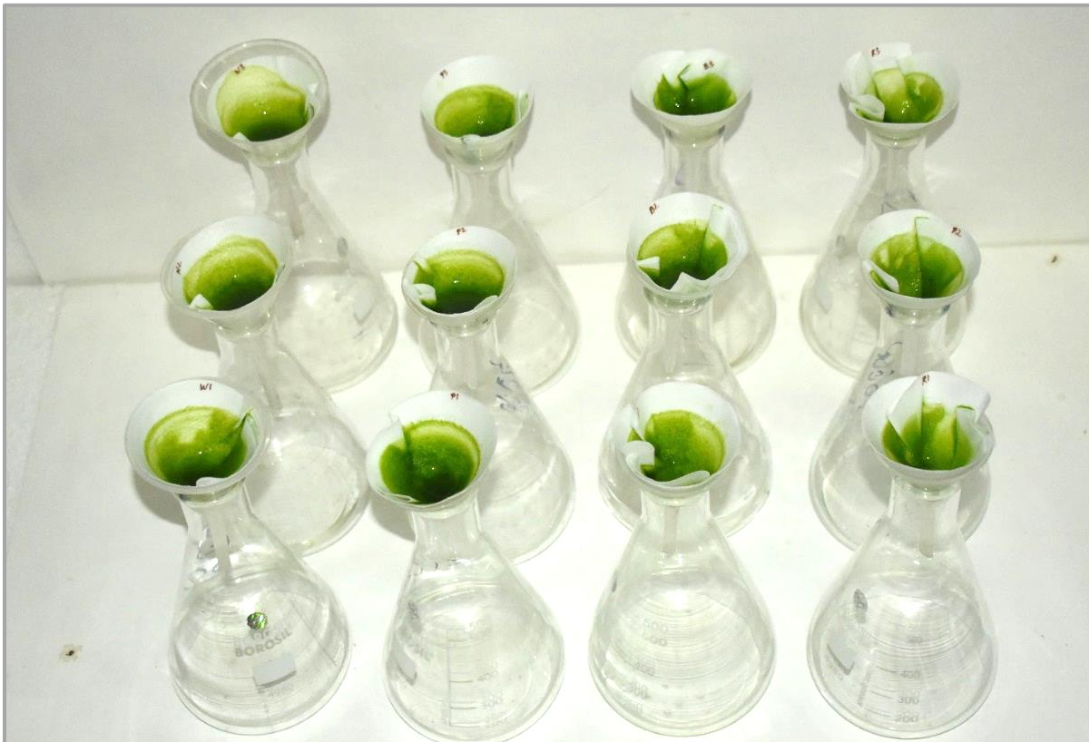
Figure 3A.21: Microalgae culture filtered using glass microfilters for microalgae growth measurement using gravimetric method.
