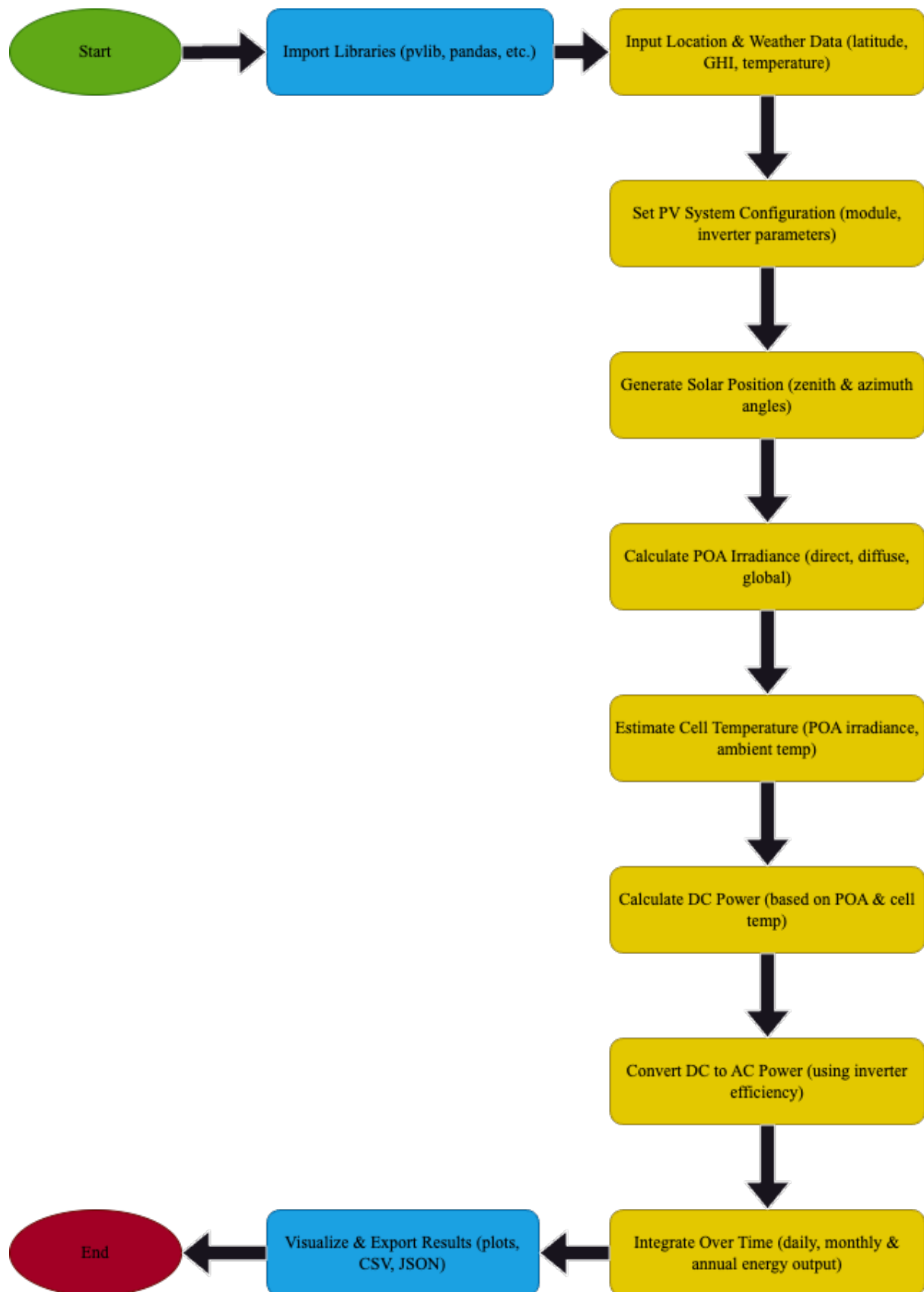
Fig 3.6: PVlib simulation flowchart: Steps for photovoltaic energy system modeling
