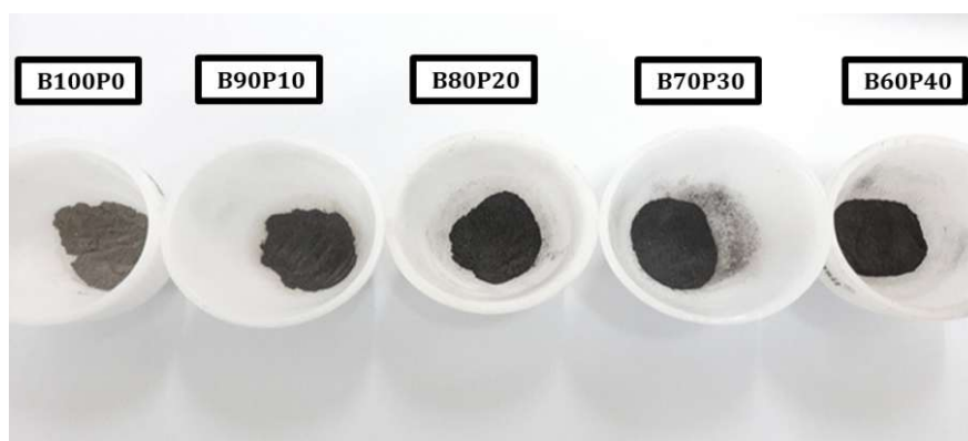
Fig. 4.8 Ash residue of blended fuel particles
