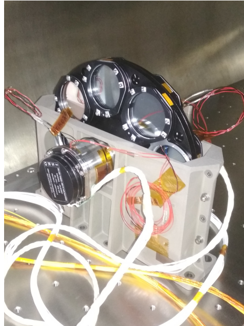
Figure 2.10: Assembled flight model of SUIT Filter Wheel Assembly [34].
