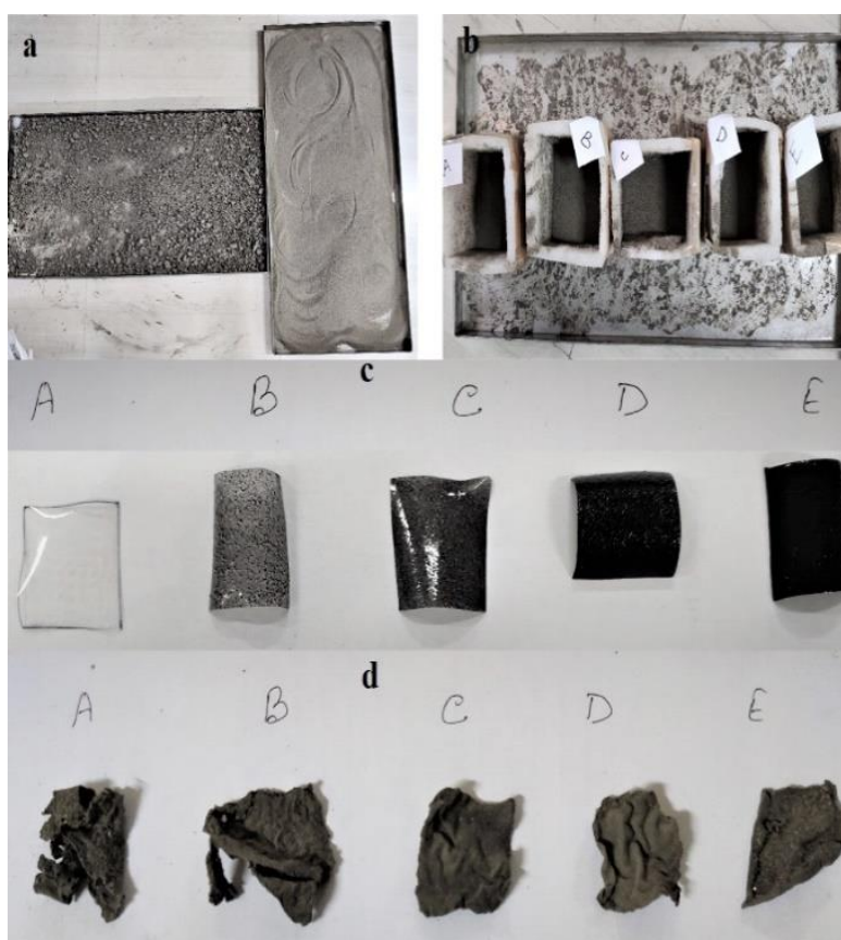
Figure 4.12 Soil burial analysis of PVA and PVA/GO films (a, b) soil preparation (c) samples (3×3 cm) (d) 20 th day sample degradation
