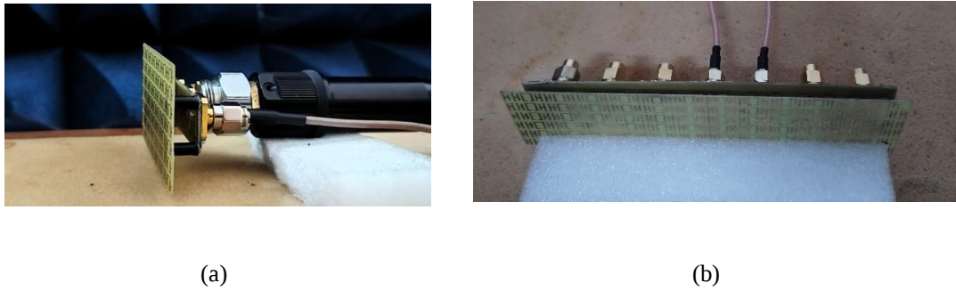
Figure 6.2 Proposed metasurface for mitigating mutual coupling in closed spaced (a) 1 \times 3 and (b) 1 \times 7 patch antenna array.
