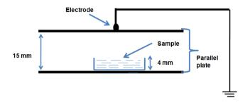
Figure 3.2 Cold Plasma Parallel plate attachments
