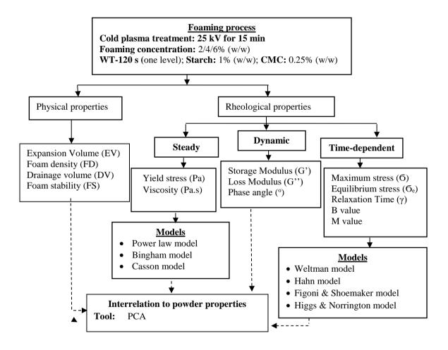
Figure 3.4 The schematic diagram of a methodology for objective #3
