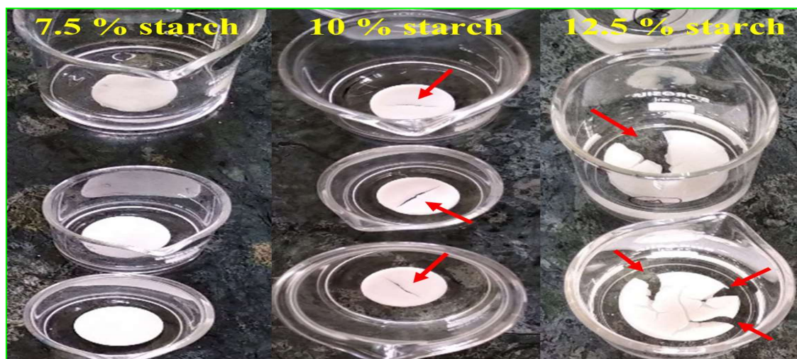
Fig. 3.2 Solvent exchange of hydrogel made of different starch concentrations
