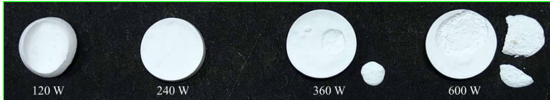
Fig. 4.1 Developed aerogel through microwave drying at different power level
