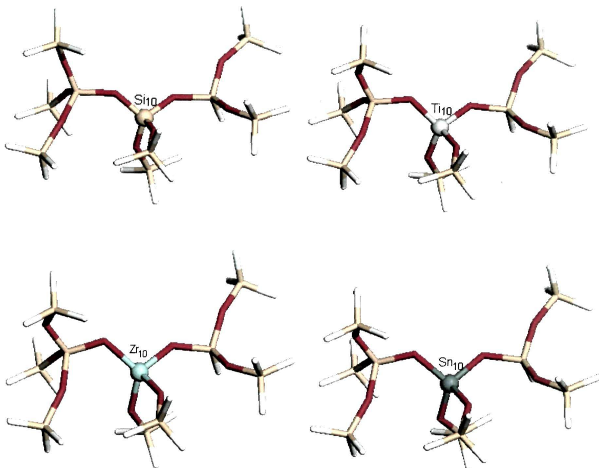
Figure 5.2: Optimized T10 site of purely siliceous, titanium, zirconium and tin substituted 10T cluster of MFI zeolite. The dangling bonds are saturated by hydrogen atoms
