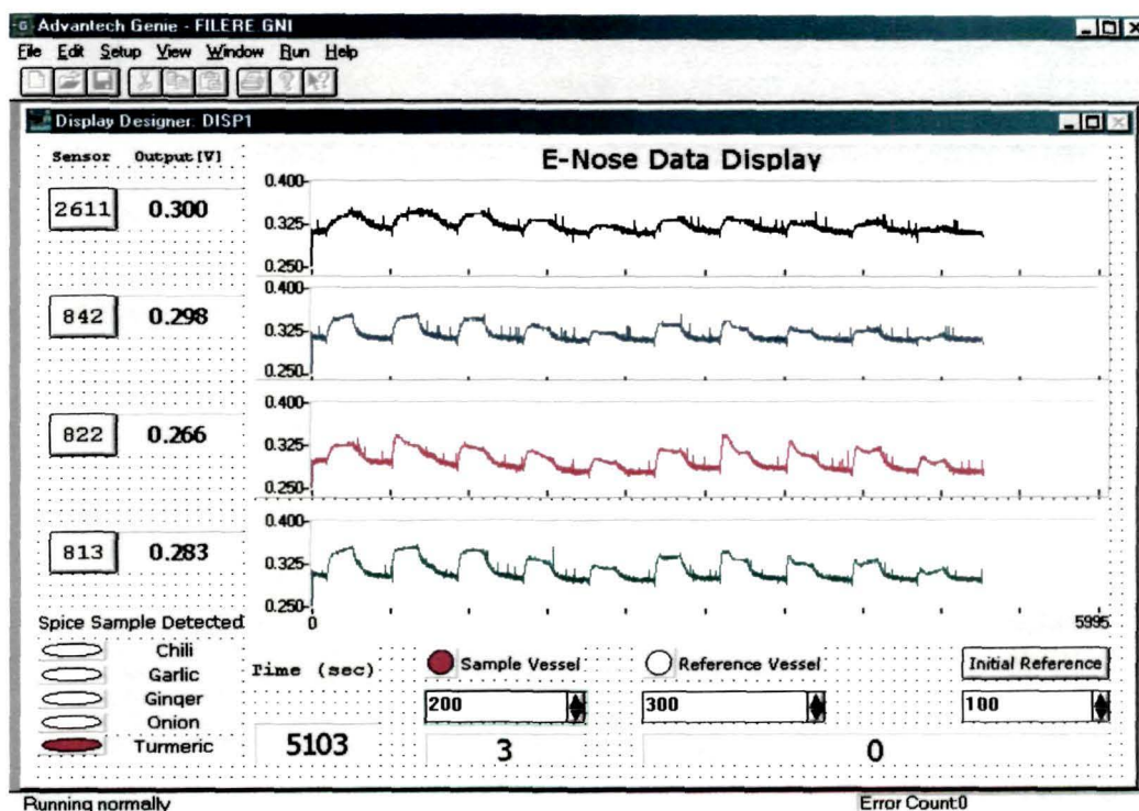
Figure 4.16: A typical response of E-nose sensors to the sample of turmeric spice in an experimental process.
