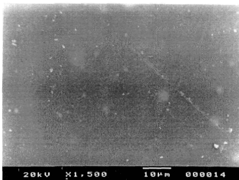
Fig.4.7c. SEM micrograph for the composition 0.019 \text{ PSBUAMVSB} : 6.5 \times 10^{-3} \text{ TEOS} : 2.95 \times 10^{-3} \text{ HCl} : 0.123 \text{ THF}
