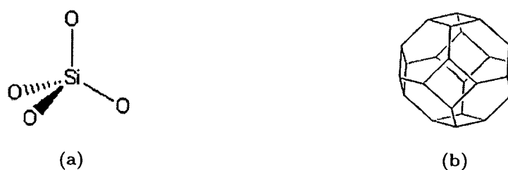
Figure 1.7: Structures of (a) primary building block, \text{SiO}_4 tetrahedra and (b) secondary building block, sodalite cage of zeolites.
