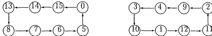
Figure 2.5: The state transition diagram of a nonmaximum length group CA
