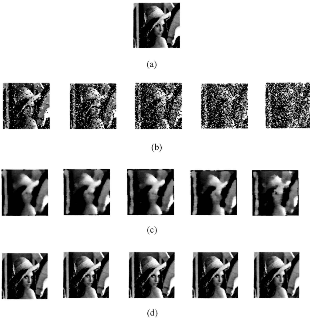
Figure 7.11. (a) Original 512 X 512 Lena Image cropped into 80X80 size, (b) Original Image of (a) corrupted with noise density of 10%, 20 %, 30%,40%, and 50% respectively, (c) Image after median filtering of mask 3x3, (d) Restored image using proposed MED-BFO technique.
