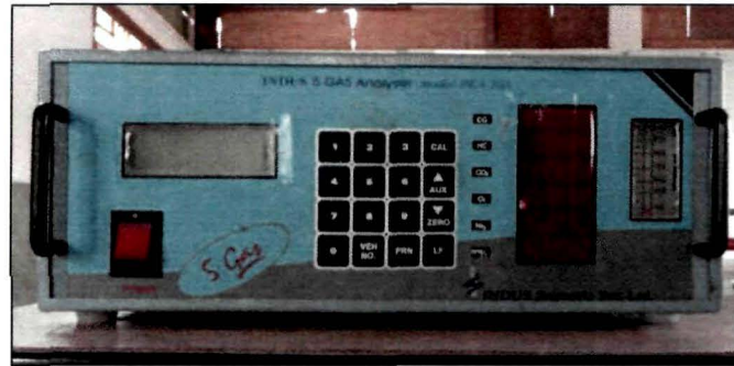
Fig 3.13 Laboratory exhausts gas analyzer
