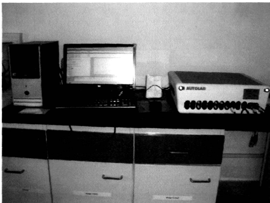
Figure 4.6: Potentiostat/galvanostat along with PC control for IV characteristics of fabricated OPV devices.
