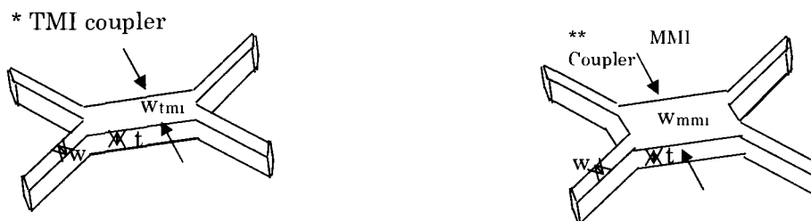
Fig-2.5: Different device structures (a) cross section of DC with embedded rectangular waveguide (b) DC with Rib waveguide (c) DC with Ridge waveguide (d) TMI coupler (e) MMI coupler
