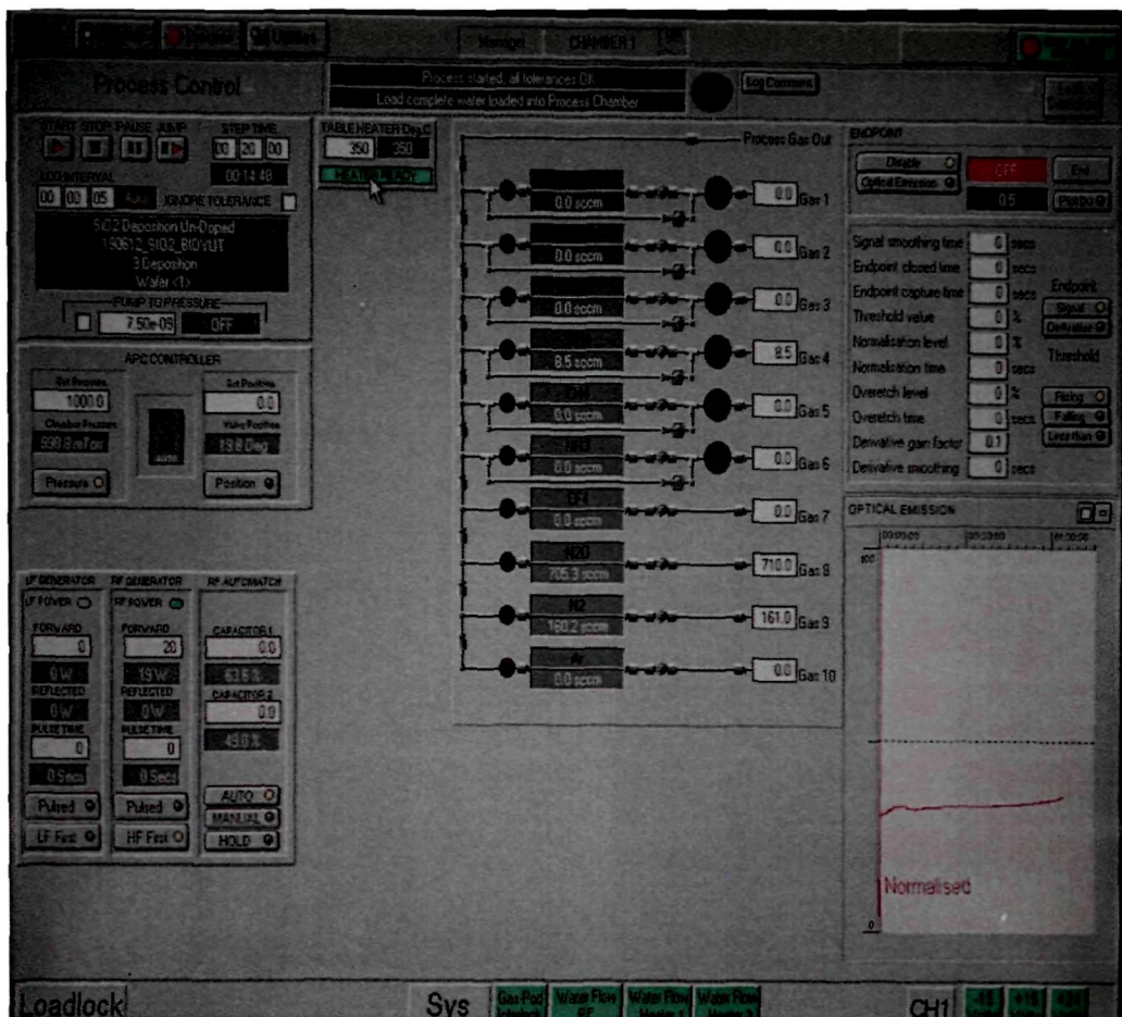
Fig-6.15: Process parameters for deposition of SiO 2 layer using PECVD
