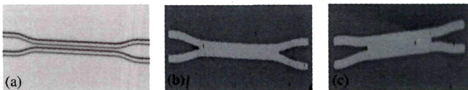
Fig-6.33: Microphotograph of successful lift-off structures (a) DC, (b) TMI coupler and (c) MMI coupler
