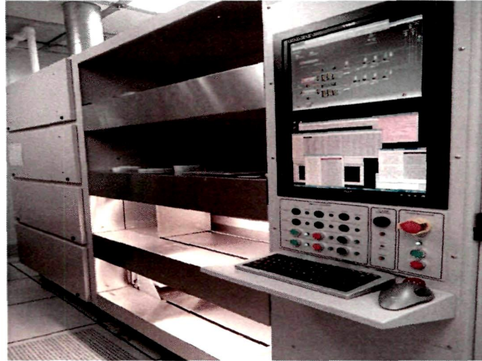
Fig.-6.23: First Nano Drive-in Furnace (Installed at CeNSE, IISc.)
