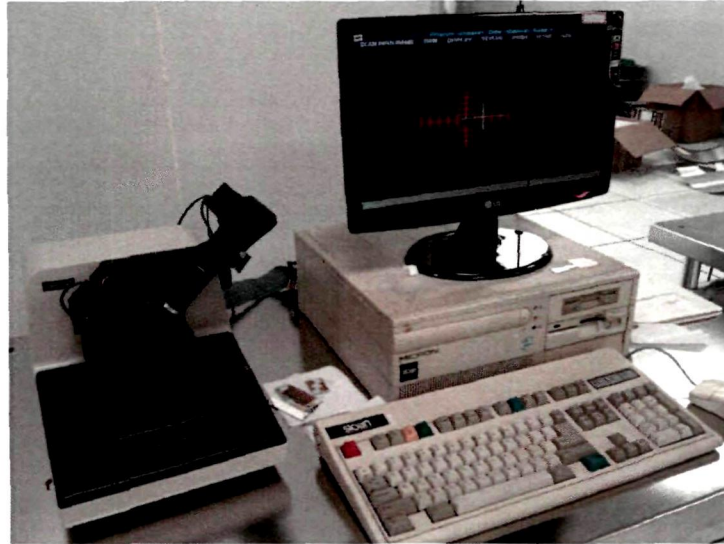
Fig.-6.36: Dektak Set-up for step height measurement (CeNSE, IISc.)
