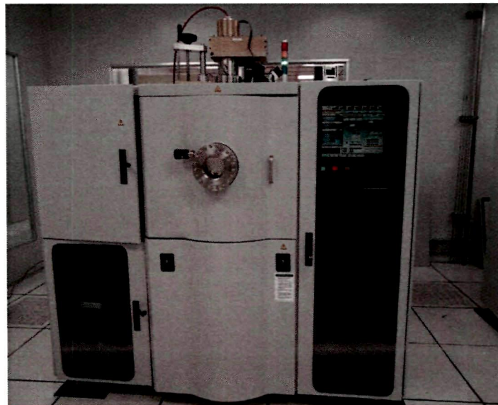
Fig.-6.30: RF sputtering unit (Installed at CeNSE, IISc.)
