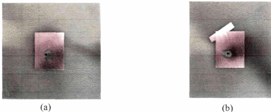
Figure 4.17: (a) Fabricated simple patch designed at 4.75 GHz
