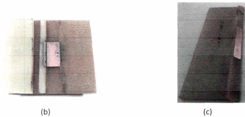
Figure 3.33: (a) Isolated substrate section before adding to elevated patch section (b) Fabricated elevated section before addition ( \theta_e = 45^\circ ) (c) Isolated substrate section added to elevated patch section
