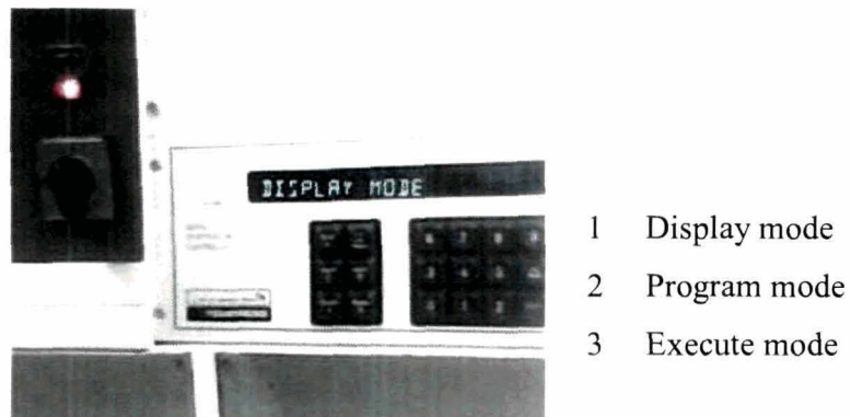
Fig-3.11: Digital temperature controller
