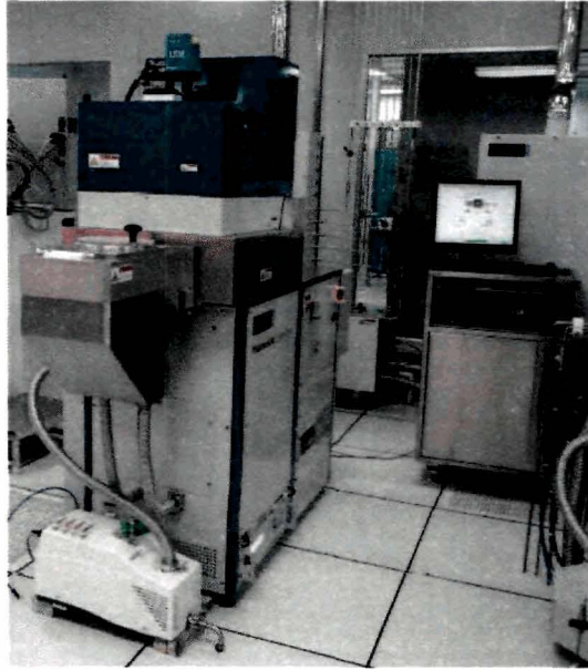
Fig-3.36: RIE Set-up, F based (PlasmaLabSys-Oxford Instrument System), CeNSE
