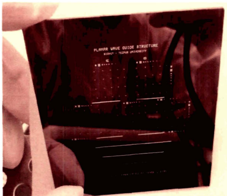
Fig.-3.25: Patterned Mask for Photolithography
