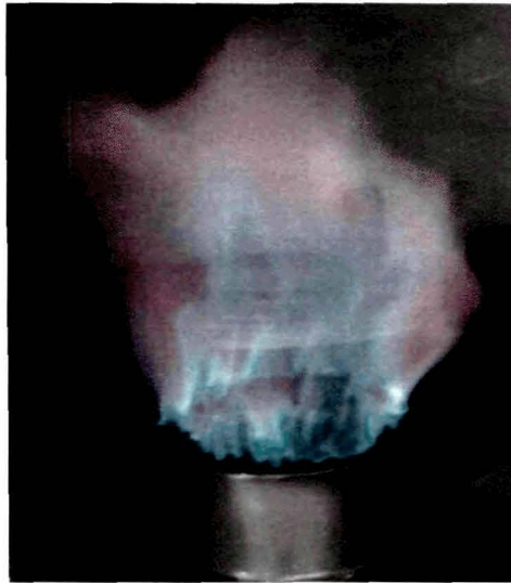
Fig.4.1d Producer gas flame ( \phi = 0.7 )
