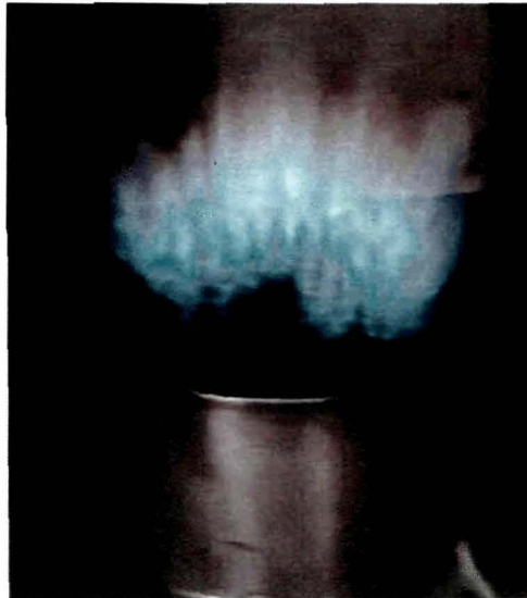
Fig.4.1f Producer gas flame ( \phi = 1.1 )
