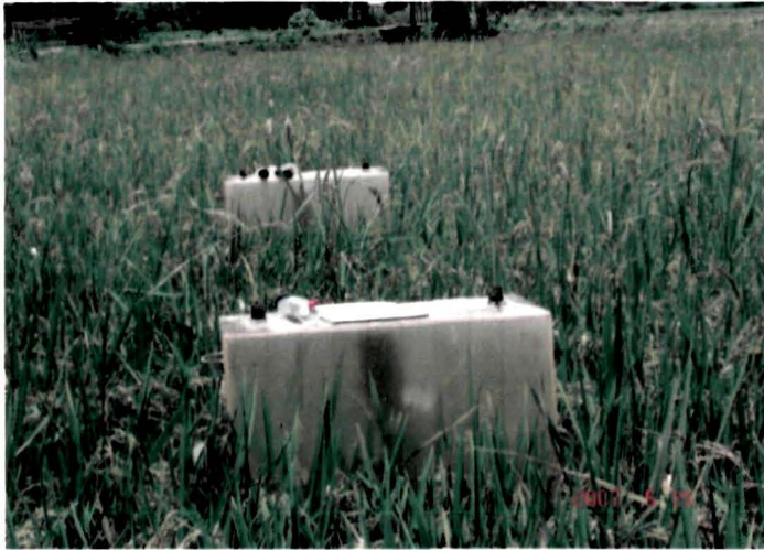
Plate 3.1. Gas sampling in rice field by static chambers
