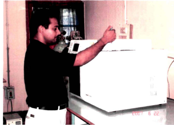
Plate 3.2. Gas-sample analysis in Gas Chromatograph
