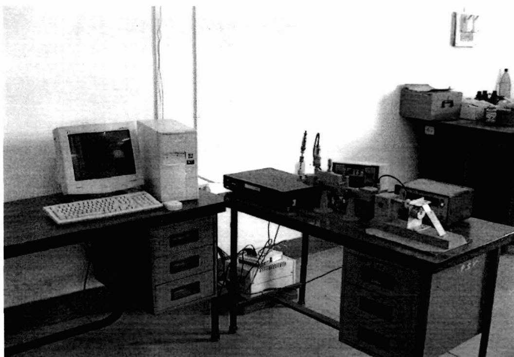
Figure 2.7. Photograph of fully computerized Microwave X-band measurement Setup
