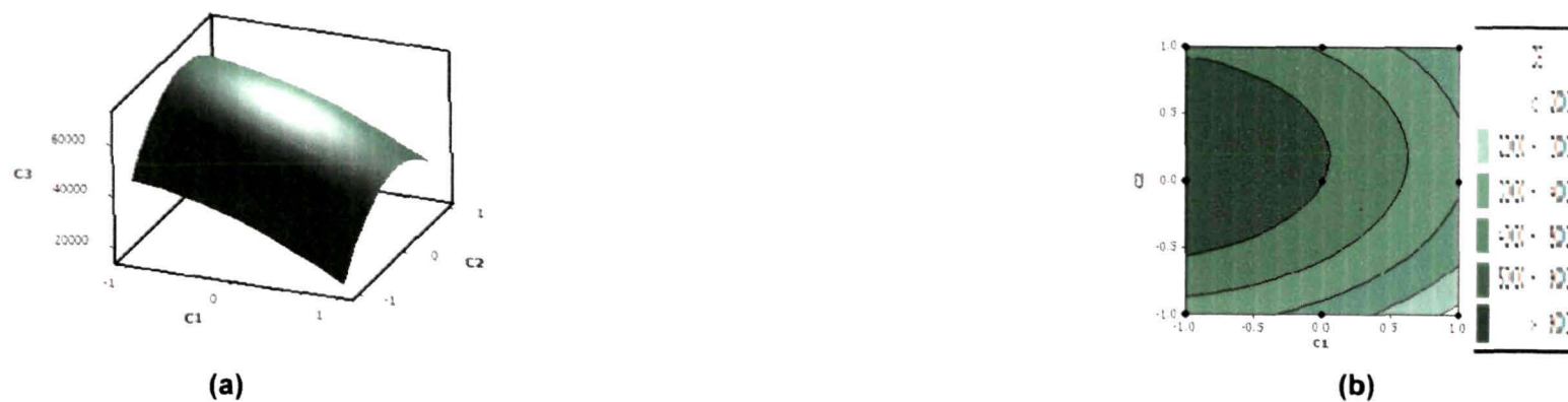
Fig.7.29 Legend shows response surface plot (a) and contour plot (b) of specific activity of iron-oxide MNP bound \beta -keratinase vs pH of buffer (Tris-HCl) system used. C_1 , amount of MNP (in coded value), C_2 , pH of Tris-HCl (in coded value), and C_3 (specific activity in U/ mg).
