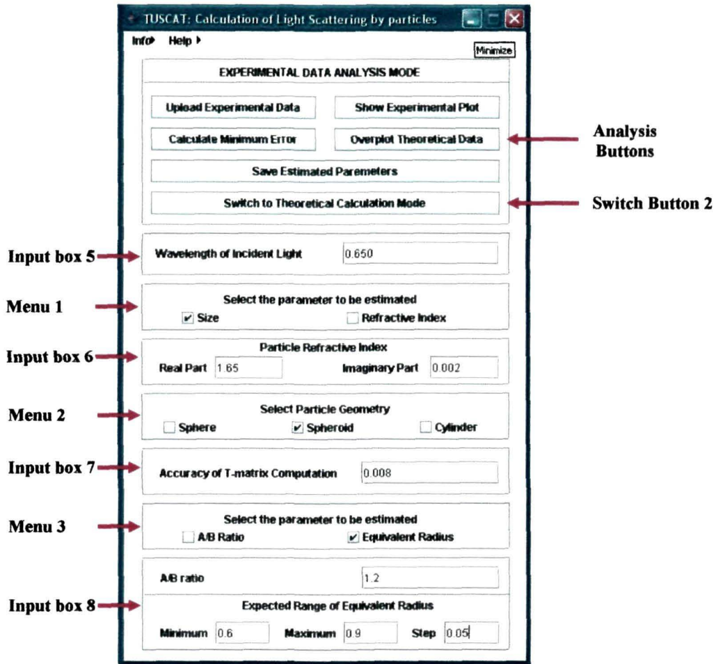
Figure 3.27. Screenshot of the control panel in the ‘Experimental Data Analysis Mode’ of TUSCAT for size estimation.
