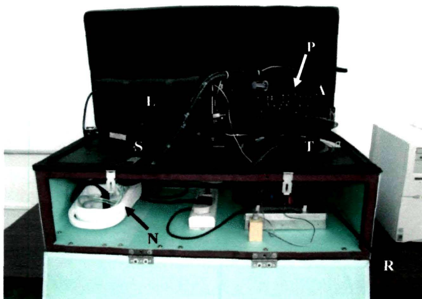
Plate 3.1. A photograph of the light scattering setup. L: laser source; S: mechanical jack; N: nebulizer for spraying water droplets; T: turn table; A: detector array; P: aerosol nebulizer; R: external rack.
