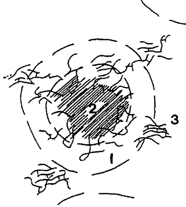
Figure 2.8: Schematic drawing of morphology of composite polymer–nonconductive filler electrolytes. Numbers are attributed to (1) highly conductive interface layers coating the surfaces of grains, (2) dispersed insulating grains, (3) matrix polymer ionic conductor [238].
