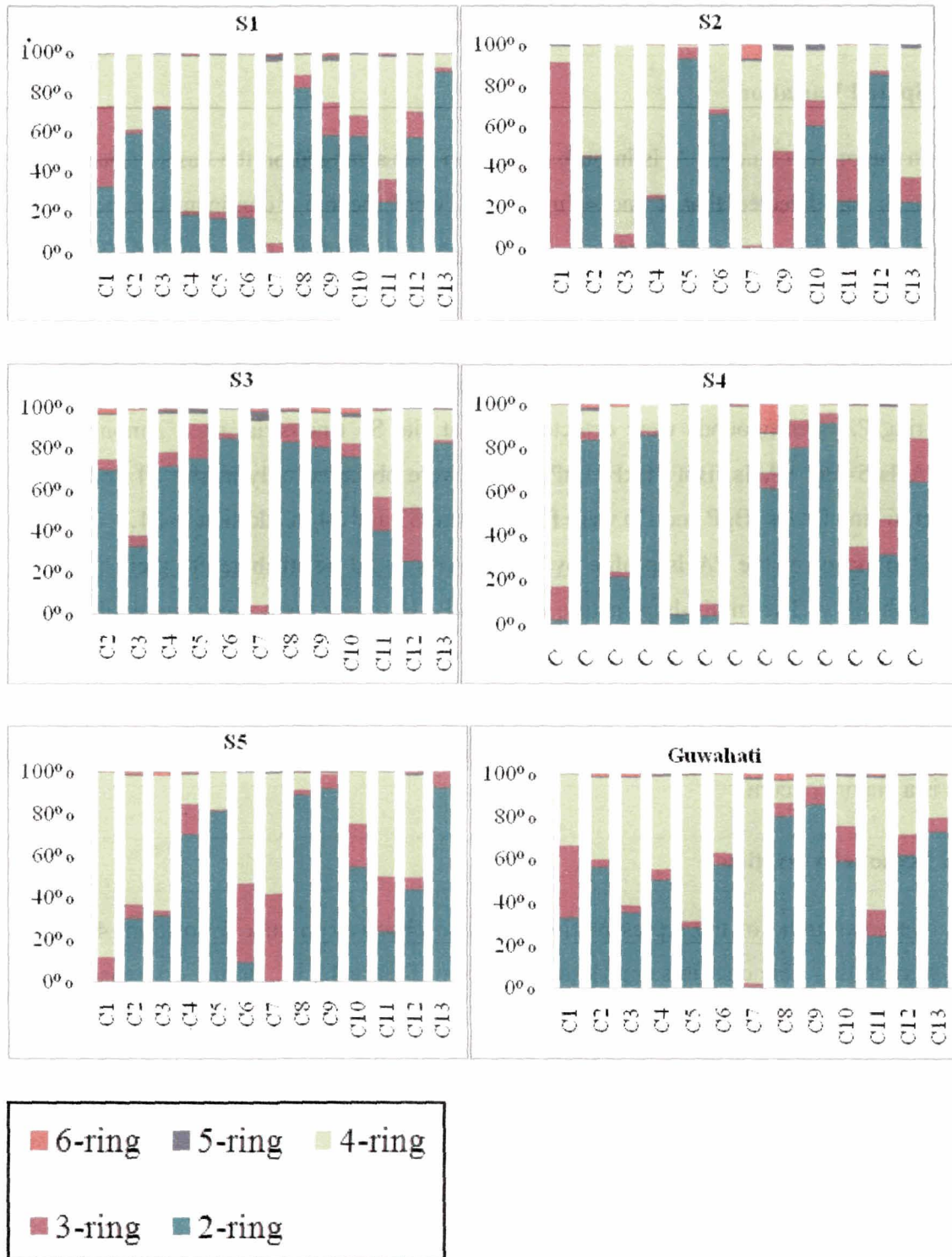
Figure 4.2.a: Percentage composition of three-, four-, five- and six-ring PAHs at sampling sites (S1-S5 and mean of the five sites as Guwahati) in bulk deposition samples (C1-C13 are sampling events from February 2011 to February 2012).
