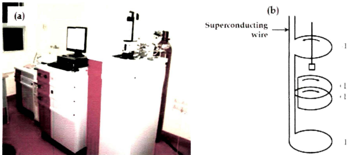
Figure 3.11: (a) SQUID magnetometer (Quantum Design: MPMS XL-7) used for magnetic property measurements and (b) schematic of superconducting coil through which sample is scanned.
