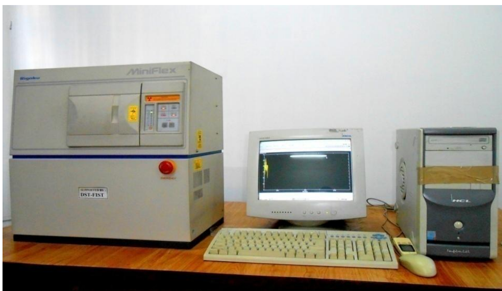
Figure 3.5: X-ray diffraction measurement unit (Rigaku, MiniFlex).
