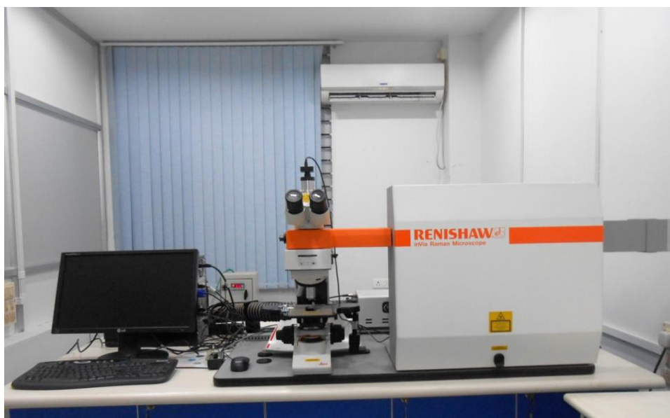
Figure 3.8: Photograph of micro-Raman spectrometer (Renishaw in-via).
