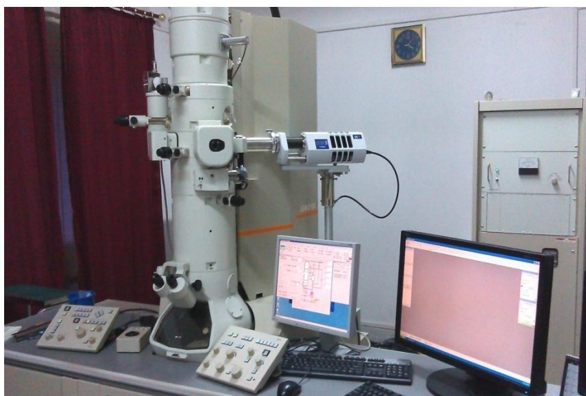
Figure 3.4: High resolution transmission electron microscope (JEOL, model JEM-2100).
