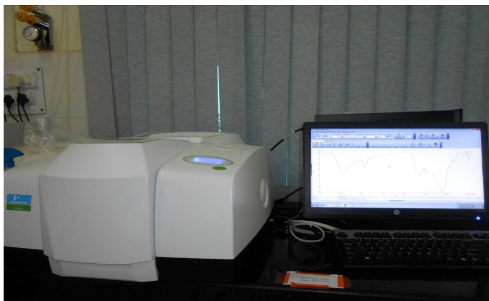
Figure 3.7: Photograph of FTIR spectrometer (Perkin Elmer, model spectrum 100).
